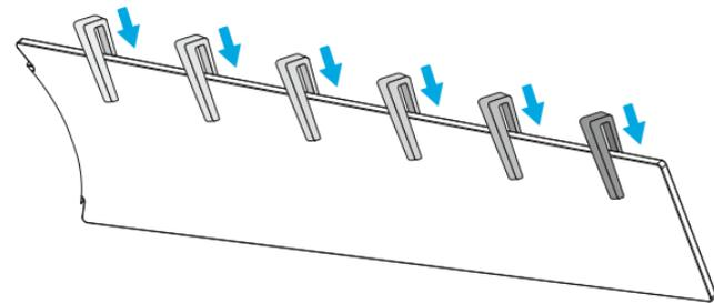
Now, move the clip to the blade that caused the least wobble. Run your fan and observe the wobble. Adjust the clip in small increments along the edge of the blade to achieve the least wobble.
