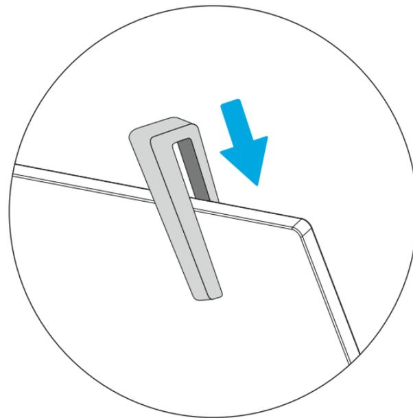
Pause your fan to attach the clip to the end of any blade. Run your fan and observe the wobble. Stop the fan and move the clip to the next blade, repeating these steps for all the fan blades.
