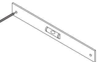
2. Drill holes for included anchors. Insert included anchors and screws.
